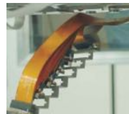
Circuits made of DuPont™ Pyralux®, like ones for the Mars Exploration Rover's panoramic cameras.
